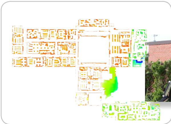
Northwood-Kensett High School - left to right: 2D floor plan created by TIMMS; TIMMS in front of School and LiDAR overlay of class room.
